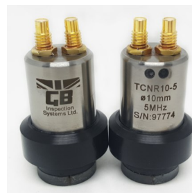
TCNR Twin Crystal Track Network Rail Approved Version Twin Crystal 0° Normal Beam Crystal Size: 10mmø
